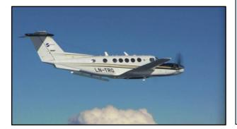
Name: Beech King AIR B200 Manufactor: Beechcraft Engine: 2 x Pratt & Whitney PT6A-42 Length: 13,36 Wing span: 16,61 Height: 4,52 Maximum weight:5.670 Maximum speed: 546 Cruise Speed: 535 Range: 3.095 km Max Altitude: 10.668 m Crew: 2-4 depending on task
