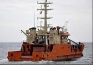
Name: Mette Miljø, A562 Call sign: OUEB Homeport: Frederikshavn Length: 29,75 m Width: 8,02 m Draught: 2,0 m Gross Tonnage: 247 tons Mast Height: 14,7 m Power (KW): 485 KW Bollard pull: ? Max Speed: 9 knots Range: 1000 Nm Minimum crew: 6 (total berth capacity) Mobilisation time: 2 hours
